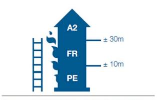
As soon as the building is higher than the firefighters' ladders, it has to be conceived with an incombustible material.
