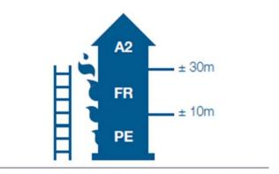
As soon as the building is higher than the firefighters' ladders, it has to be conceived with an incombustible material.
