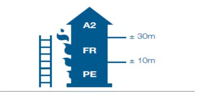
As soon as the building is higher than the firefighters' ladders, it has to be conceived with an incombustible material.
